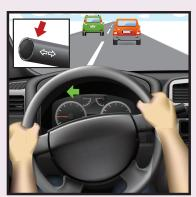
FEATURE DOES NOT ALERT DRIVER WHEN THE TURN SIGNAL IS ACTIVATED
