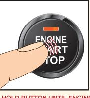
PUSH AND HOLD BUTTON UNTIL ENGINE STARTS OR SHUTS OFF
