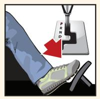
STEP ON AND HOLD BRAKE, PUT GEAR SHIFT IN PARK
