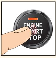
PUSH AND HOLD BUTTON UNTIL ENGINE STARTS OR SHUTS OFF
