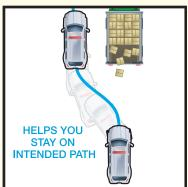
ESC WORKS BY BRAKING INDIVIDUAL WHEELS AND REDUCING ENGINE SPEED – HELPING YOU MAINTAIN CONTROL.
