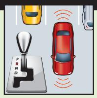
SHIFT INTO REVERSE TO ACTIVATE THE FRONT AND REAR PARKING SENSORS
