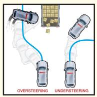
ESC ENGAGES AUTOMATICALLY TO PREVENT OVERSTEERING AND UNDERSTEERING.
