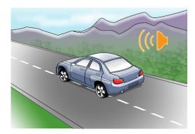
Some vehicles are equipped with lane keeping assist, which is a more advanced version of lane departure warning. If the system detects a potential lane departure and you do not respond in time, lane keeping assist will gently steer you back into the lane.
