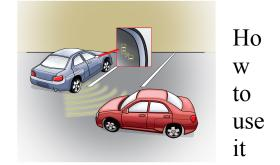
When backing out of a space, reverse slowly. The rear cross traffic alert system will alert you when other vehicles are detected near or in your backing path. Once the rear end of your vehicle is beyond adjacent objects and vehicles, the rear cross traffic alert system will then have a clear view of traffic approaching from the left or right. When using rear cross traffic alert, you must always check over your right left shoulders and be cautious when backing up.
